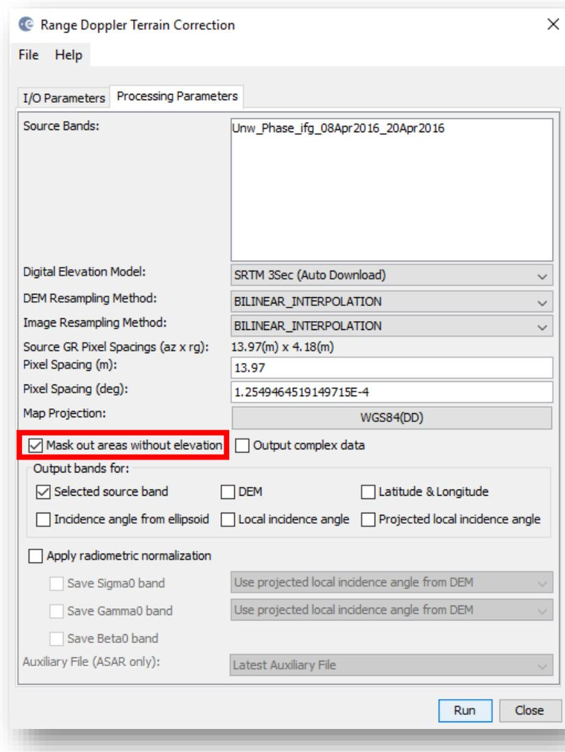
**Figure 11: Range Doppler Terrain Correction**
