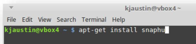
**Figure 4.** At the Linux command line, install SNAPHU.
