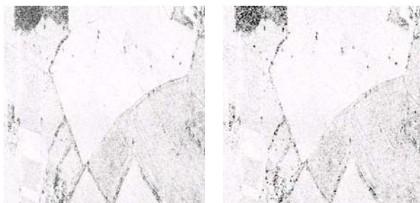
Figure 2 Left: Monks Wood interferogram coherence; right: correlation coefficient of image intensities converted to a coherence
